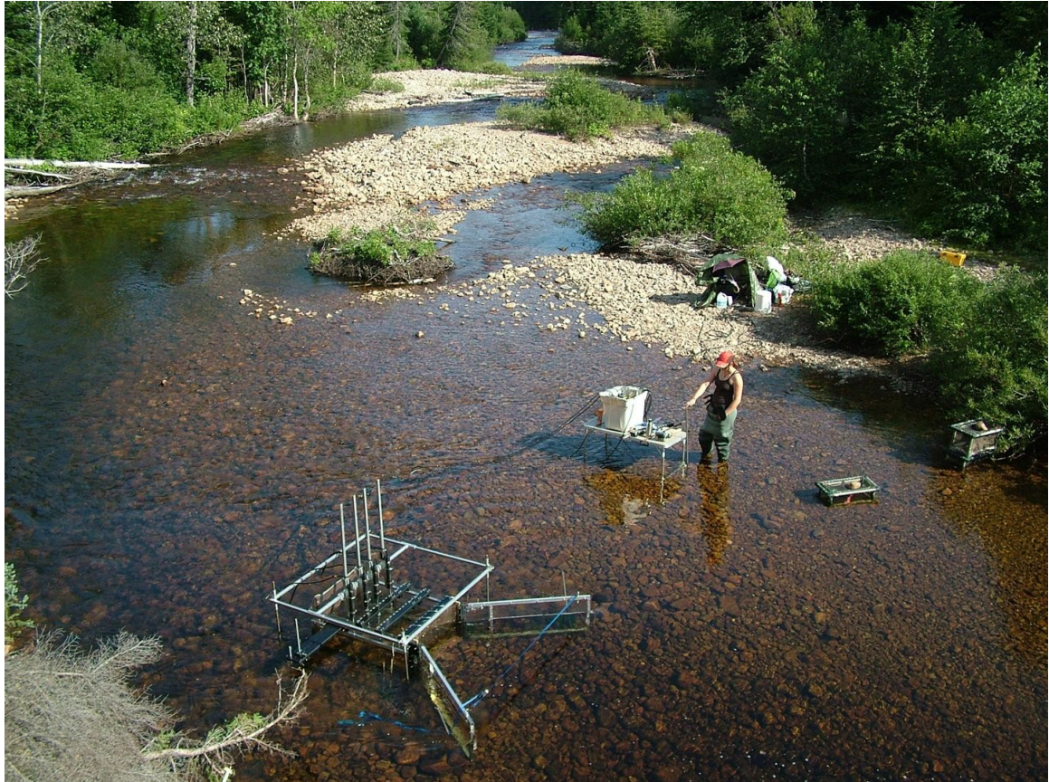
Figure 3.6 Portable flume installed in the ‘open’ doors position in Xavier Brook, Saguenay in the summer 2009. Superimposed aluminum graduated frame holds acoustic Doppler velocimeters.
