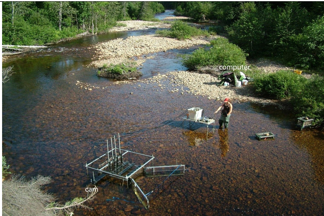
Figure 5.3 Portable flume installed in Xavier Brook. Camera and velocity probes were wired to a computer on the bank. Four Acoustic Doppler velocimeters (ADV) were used to characterize hydraulics within the observation section. ADVs were removed during feeding trials.
