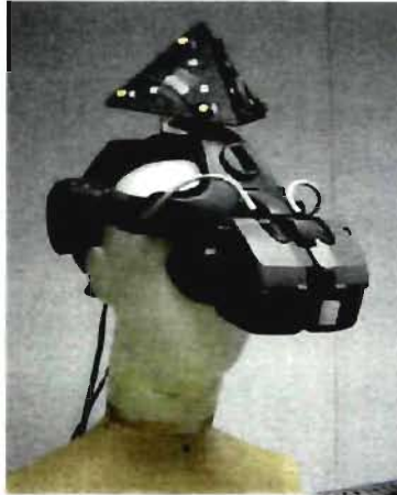
Figure 5. HMD used to display the VE to the user; and the rigid body with the IREDs used to reproduce the position and orientation of the head in the VE.
