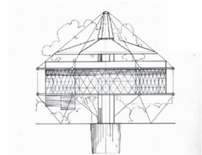
Figure 23 : La Dymaxion House et le principe de Tensegrity : source [http://www.trackchanges.net/wp-content/uploads/2008/09/dymaxion.jpg]
