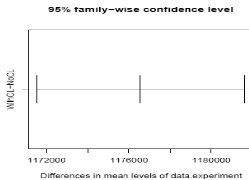
Figure 4.17: Turkey HSD showing the difference in average bandwidth between NoCL and WithCL.
