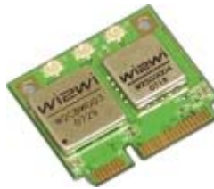
Figure 1: Circuit card with 3 fully integrated radio technologies [21]
