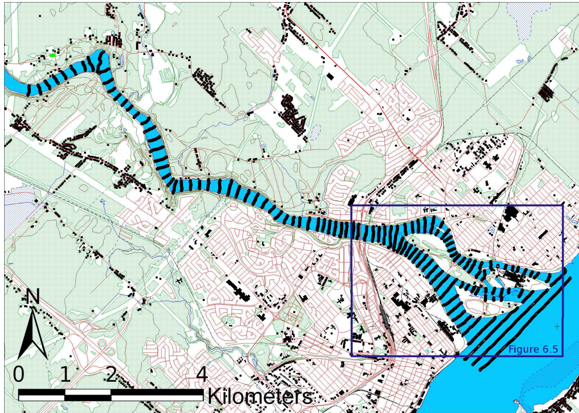
Figure 6.4: The Saint-Maurice River with the measured cross sections.
