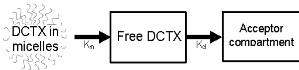
Figure S1. Kinetic model for DCTX release from micelles in jacketed Franz diffusion cells.
