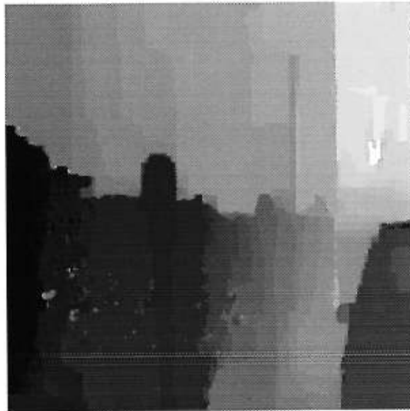
Figure 8.22. Disparity maps for the Park meter. Results are shown for 4 image sequence. The matching volume is 256x240x64.
