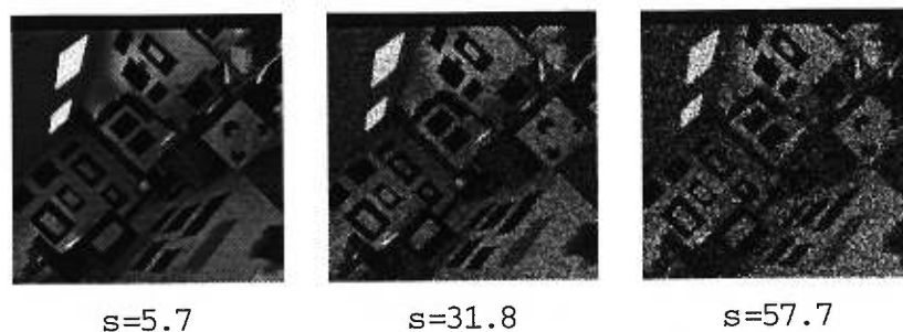
Figure 4.10. Image degraded by uniform noise. "s" is the standard deviation of the noise.
