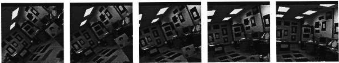
Figure 4.7. The Puma image sequence, frames 1,4,7,10,13. The camera is at the end of a Puma robot arm rotating around its elbow in increments of 4^\circ .
