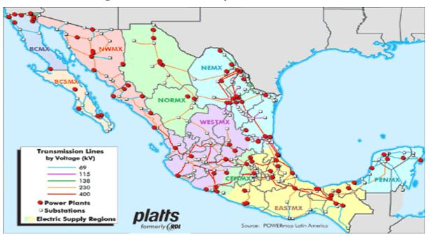
Figure 4: Mexican electricity transmission network
