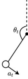
Fig. 4.3. Sketch of the pendulum-v0 task as described in the OpenAI gym documentation . The action is a torque applied to the simple pendulum, and the state space is described as the angular position \theta_t and the angular momentum \dot{\theta} .
