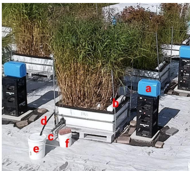
Figure 4. Aerial photos of the experimental setup taken in August 2019. Top: Aerial view of the experimental setup. IN1: inflow tank 1; IN2: inflow tank 2. Bottom: Close-up view of a mesocosm. A: 20 L influent container; B: Perforated water inlet pipe; C: Water outlet valve for sampling and draining of the mesocosms; D: Overflow; E: 20 L bucket; F: 10 L bucket for combined overflow sample collection.
