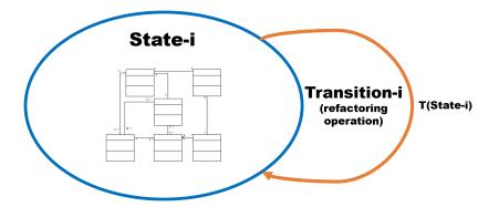
**Fig. 5.3.** Formulate the metamodel refactoring approach as an ordered Finite State Machine (FSM)
