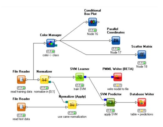
Fig. 2.15. Data flow example built with KNIME workbench source: Berthold et al. [19]
