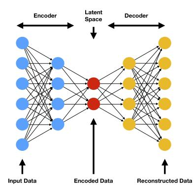
Fig. 3.13. Autoencoders architecture
