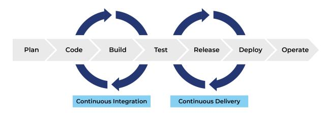
Fig. 3.8. Continuous Integration/Continuous Delivery (CI/CD) workflow
