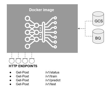
Fig. 3.5. The major components of an API template for a deployed ML model
