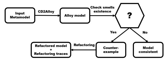
Fig. 5.1. Constraint solving approach to detect design smells and refactor metamodels
