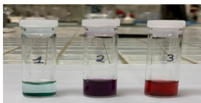
**Figure 89.** Solution color of (1)  $\text{Rh}_2(\text{OAc})_4$  (**1**) in DCM; (2)  $\text{Rh}_2(\text{OAc})_4$  (**1**) (5 mol %) and thioanisole (1 equiv.) in DCM; (3)  $\text{Rh}_2(\text{OAc})_4$  (**1**) (5 mol %), DMAP (10 mol %), and thioanisole (1 equiv.) in DCM.
