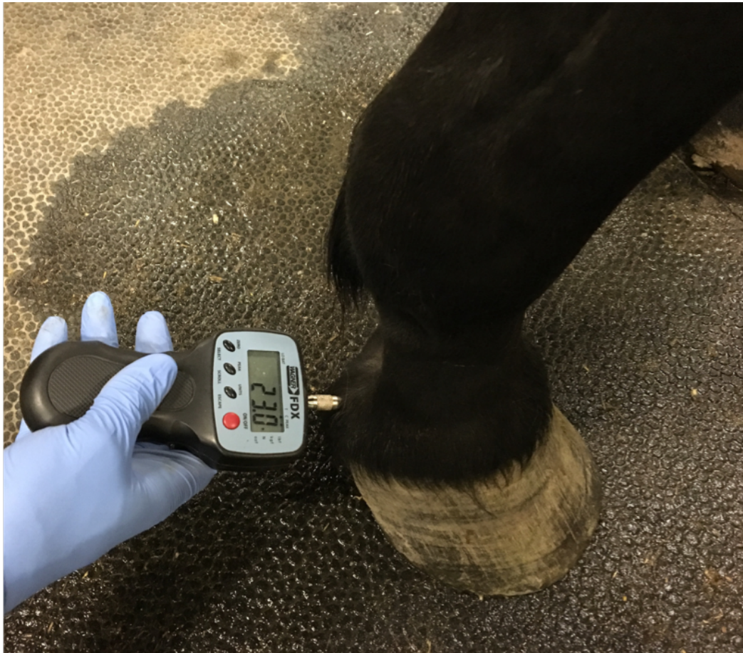
Figure 11: Image depicting the use of the dynamometer to record the mechanical nociceptive threshold at the lateral heel bulb of a right forelimb. The number displayed represents the force applied by the operator in Newtons.
