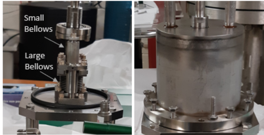
Fig. 5.2. Left: Bellows system inside of the cover regulating the pressure inside the jar during operations. Right: Close up of the top hat of the detector containing the bellows system.
