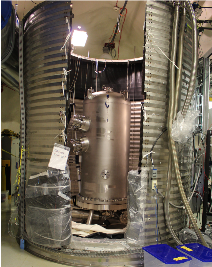
Fig. 3.3. PICO-40L detector in SNOLAB during its final installation phase. The filled C_3F_8 jar is inside the pressure vessel, which is placed inside a tank to be closed up and filled with water as a shielding against backgrounds.
