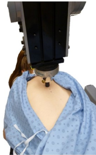
Figure 5.1. (A) Overview of the apparatus used to assess spinal stiffness with (B) a closer view of the indenter just above a participant's spinous process. The apparatus frame has been designed to move on forward and backward as well as up and down, while the treatment table was modified to allow lateral displacements.
