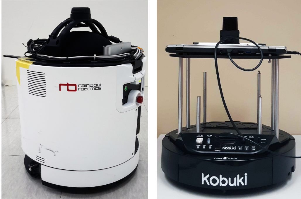
(a) JAY with top-mounted 360-degree view LiDAR (b) Turtlebot with top-mounted 260-degree view LiDAR
