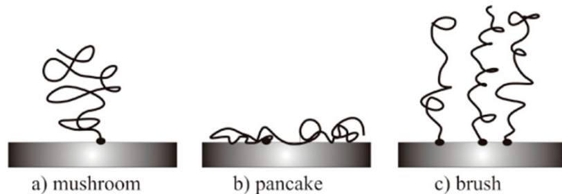
Figure 1.20. Schematic picture of three limiting structures of chemically end-grafted polymer chains. Reproduced with permission from Ref. 157. Copyright (2008), IOP Publishing.
