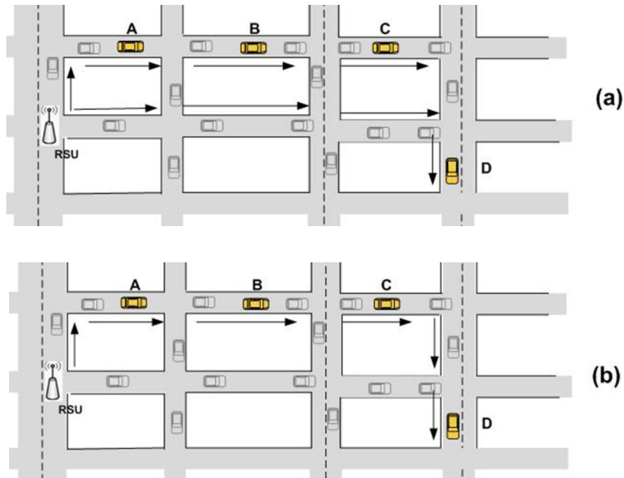
Figure 4.6 Comparison between Shortest Path Tree and Min Steiner Tree. (a) Shortest Path Tree includes 8 busy street segments, (b) Min Steiner Tree includes only 6 busy street segments.
