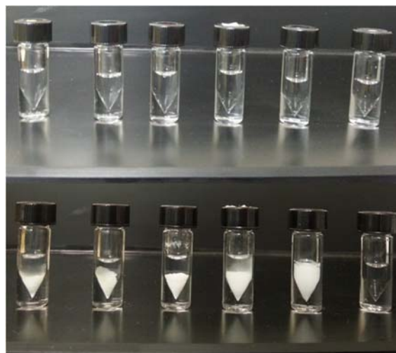
Figure SI-4. 13 Photographs of 10 g/L polymer solution before (row on the top) and after (row on the bottom) 24h of heating. From the left to the right: S-PIPOZ 1, S-PIPOZ2, S-PIPOZ3, L-PIPOZ2, L-PEG5k-b-PIPOZ2, S-PIPOZ2-b-PEG5k. The homo-PIPOZs were heated at 56°C whereas the hetero-block polymers were heated at 75°C. The photographs were taken after cooling all samples overnight at 4°C.
