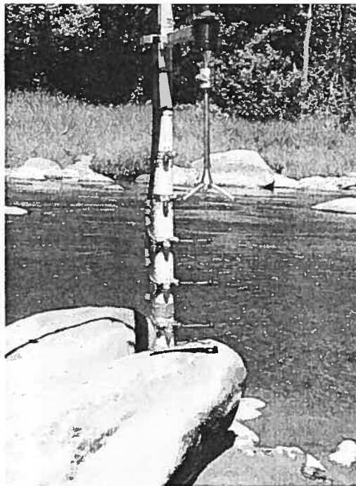
Figure 4.3 - Wading rod with ADV and three ECMs. Only the top ECM (at 25 cm) was used for this study.
