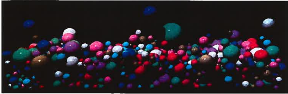
Figure 2.38 - Image of mixed sediment-size bed during modelled transport [ Schmeeckle and Nelson, 2003 ]
