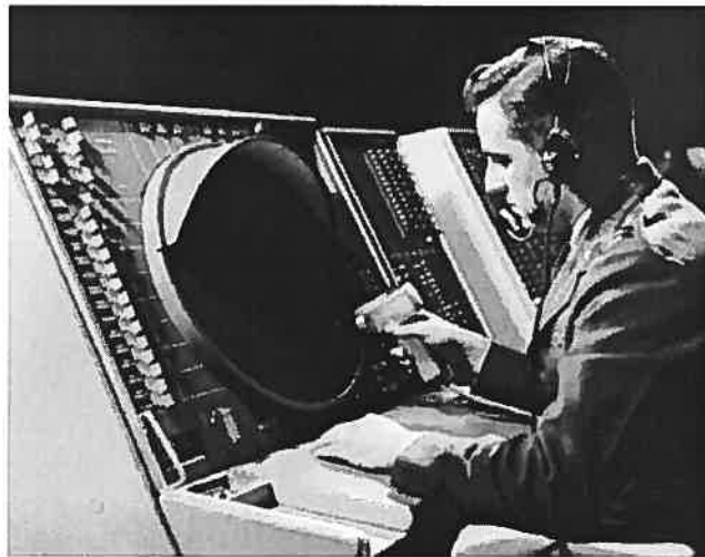
Figure 23: SAGE air-defence system light gun
