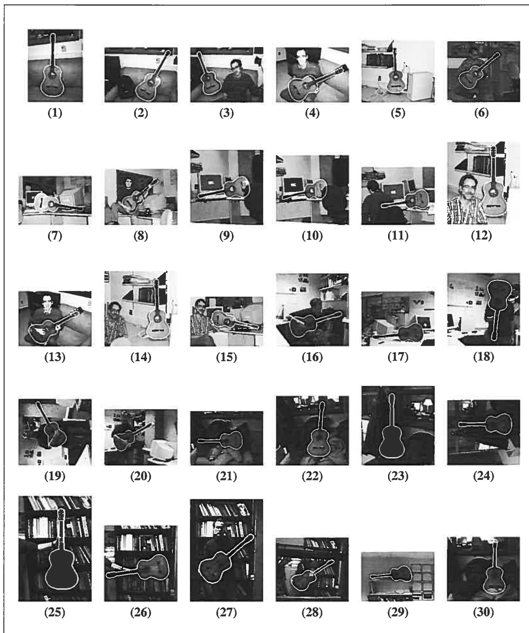
Figure 8.8. Examples of localization of a shape obtained by stochastic optimization of the Gibbs field based on the contour parameters estimated by the ICE procedure and the segmentation computed with the ESE procedure, for the guitar shape (images (1) to (30)).
