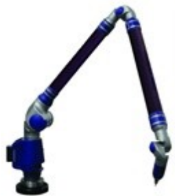
Figure 17. Bras mécanique FARO (FARO Medical Technologies, Orlando, FL, USA) 14
