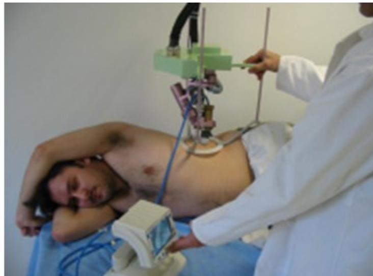
Figure 28. Le robot Otelo (mobile Tele-Echography using an ultra-Light robot) 28 .
