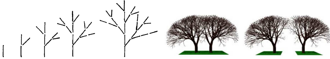
Figure 2.5: Using L-Systems for generating trees. Left: Rewriting rules for the growth of a tree [dREF*88]. Right: Growth of trees under competition for resources with an Open L-System [MP96].
