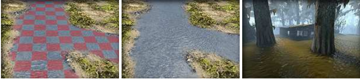
Figure 2.3: Real-time rendering of rivers using tiles of textures [vH11]. Left: The river surface is subdivided in “tiles”. Each tile has its own wave direction and speed, that are smoothly interpolated to produce the river surface animation. Middle: River with directional waves. Right: Animated marsh surface.
