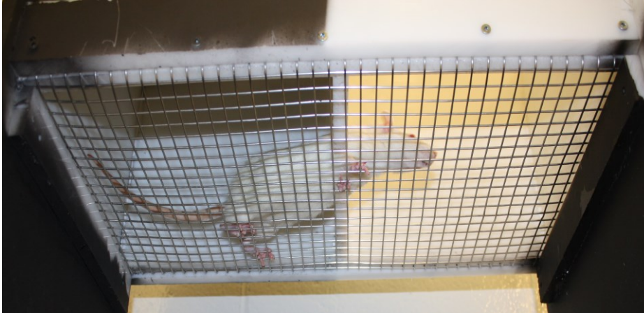
Figure 1: Picture of a rat acclimatizing to the place escape/avoidance paradigm device. The test cage apparatus was painted half white and half black and the rat was allowed to move freely from one side to another. Neither side was illuminated with additional light.
