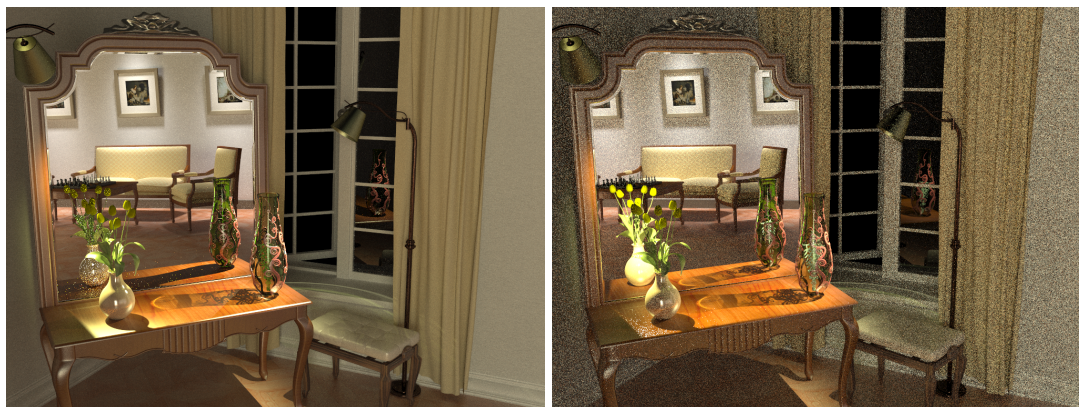
Figure 2.2: A comparison by Georgiev et al. [2012] between bidirectional path tracing (left) and stochastic progressive photon mapping (right) after 30 minutes of rendering. Stochastic progressive photon mapping produces more noisy results and cannot handle the illumination seen in the mirror. Bidirectional path tracing fails to capture the caustics of the vase reflected in the mirror.
