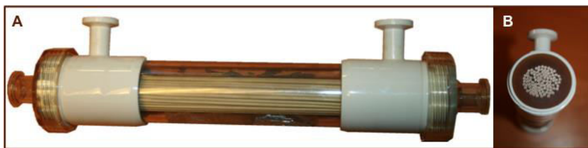
Figure S1: Hollow fiber cartridge. A. Lateral external view. B. Cross-sectional view of an end.
