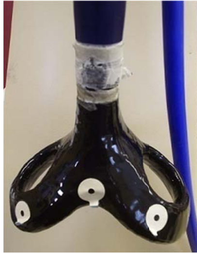
FIG. 3.3 Double-coned coil used throughout the experiments. The shape made it an ideal fit onto the subject's head and made the positioning of it easier to maintain throughout the experiment.
