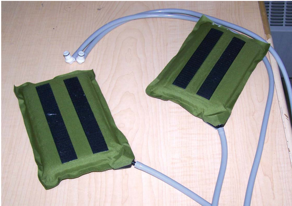
Figure 5.3 View of medium-sized air bladders, with hoses attached. These bladders were used in the work presented in Chapter 3.
