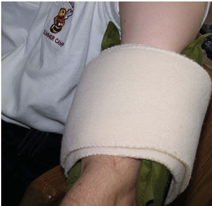
Figure 5.4 Final placement of air bladders on test subjects, secured with Velcro belt.
