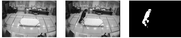
FIGURE 3.3 – Result of the moving object segmentation process. From left to right, background median model b_j , current frame i_j , segmented picture s_j for camera j .
