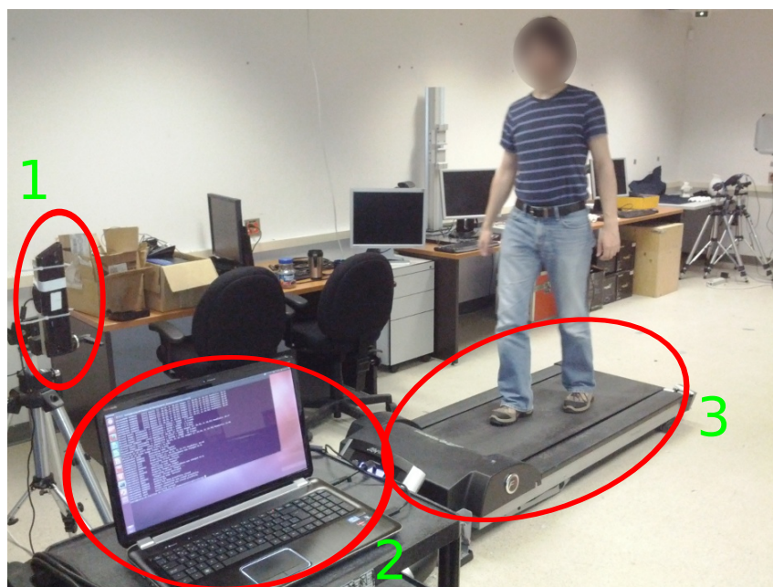
FIGURE 6.8 – Picture of the experimental setup where the depth camera (1), the recording computer (2) and the treadmill (3) are visible.
