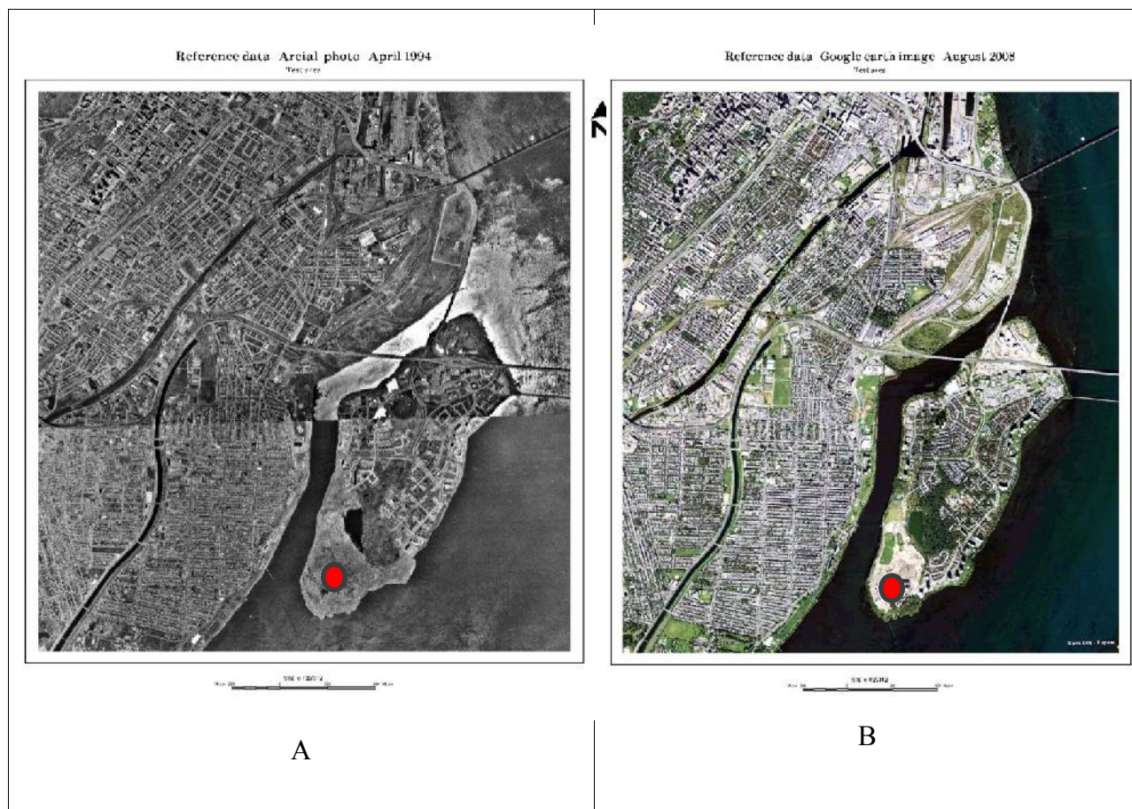
Figure 35: A: 1994 ground truth data, derived from a mosaic of aerial photos acquired in dated April 1994 B: 2008 ground truth data, derived from combining QUICKBIRD images on Google Earth acquired in August 2008
