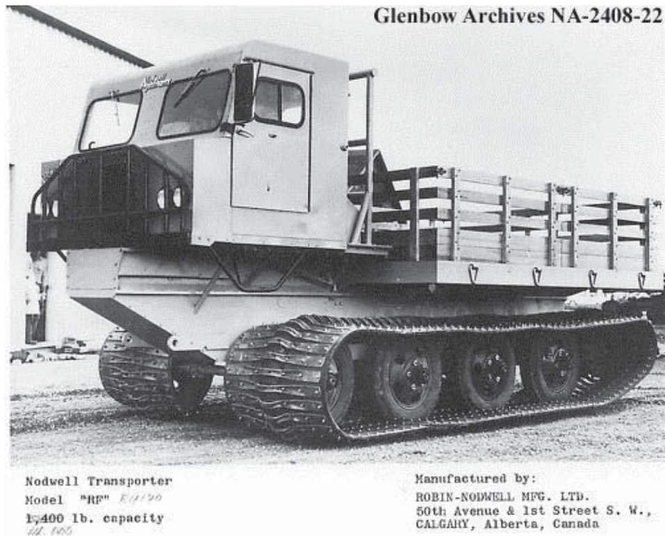
Figure 4-6. Nodwell Tracked Carrier designed by Bruce Nodwell and manufactured by Robin-Nodwell Manufacturing Ltd, 1960s model. Carrier designed to transport drill pipes in oilfield applications. Retrieved from http://ww2.glenbow.org
