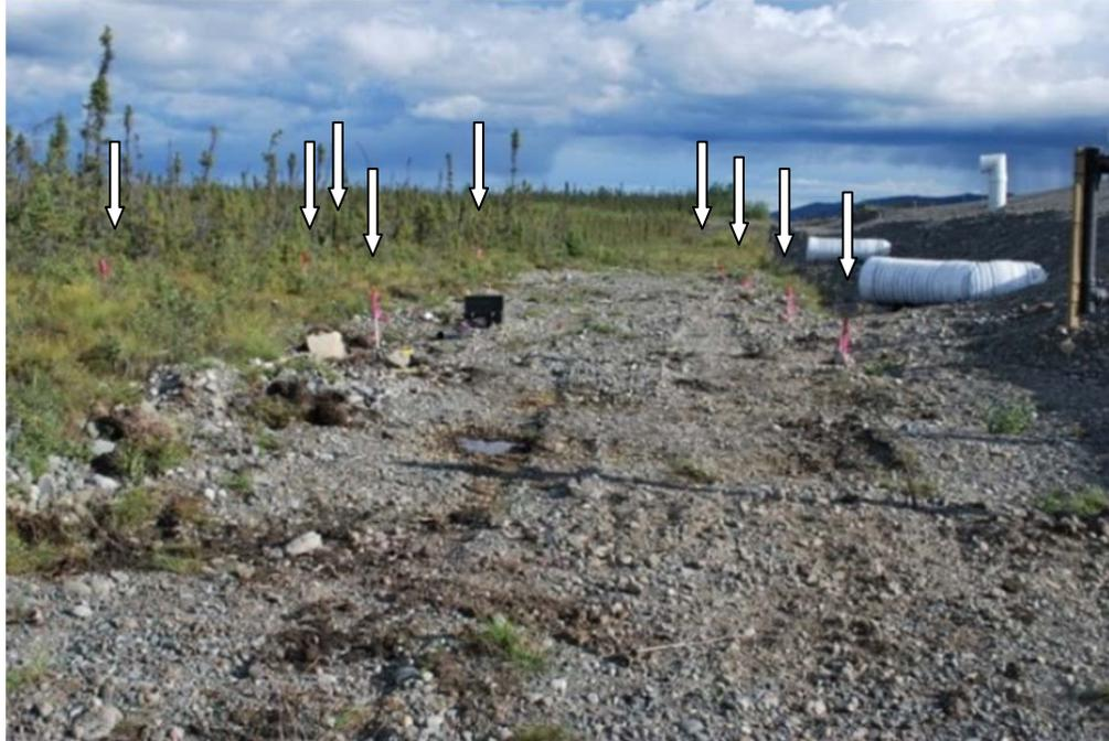
**Figure 11. Groundwater observation wells network (wooden stakes under arrows) on eastern side of the road. The white horizontal and vertical pipes in the background are mitigation measures to control permafrost degradation (see Fortier et al. for details in these proceedings)**
