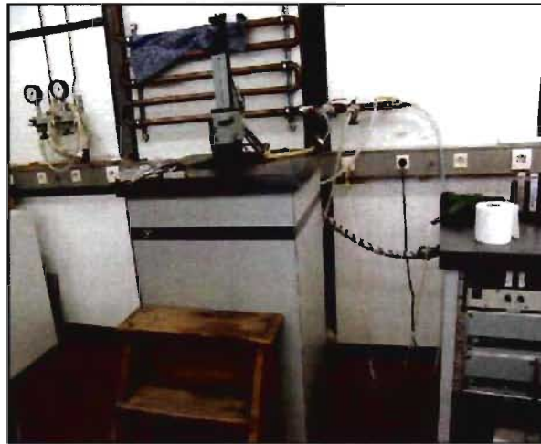
Figure 25. The picture shows the Quantum Design SQUID that was used for the measurements. With this machine, it is possible to measure in the temperature range of 4\text{K} \leq T \leq 400\text{K} and with magnetic fields up to 7 Tesla.
