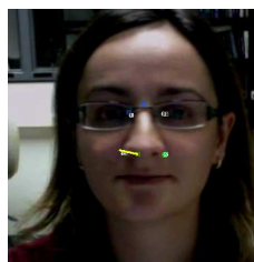
Figure B.5. A tracking failure of the nose tip affects the pose recovery.
