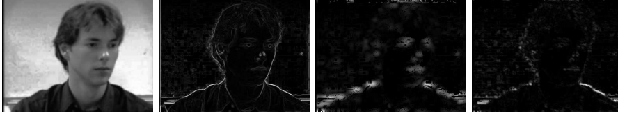
Figure C.1. Examples of the transformed images: the leftmost image is the original image; the second image represents the gradient magnitude; the two last images are the magnitude of the GWT responses for k_{1,4} and k_{4,5} respectively
