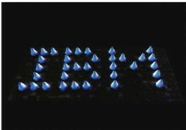
Figure 2.1 An STM image of a patterned array of xenon atoms on Ni (110). 2
