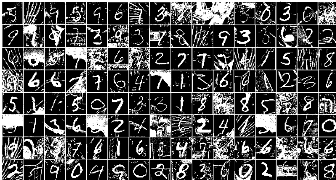
Figure 6.13: Samples from the modified MNIST digit recognition dataset with a background containing image patches. Here, a black pixel corresponds to an input value of 0 and a white pixel corresponds to 1 (the inputs are scaled between 0 and 1).
