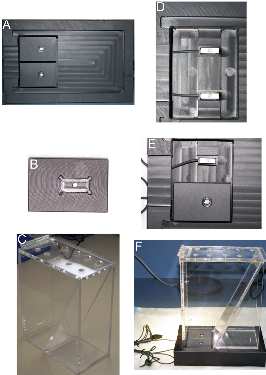
Figure 3.5: Static weight bearing apparatus assembly. (A) assembled base plate; (B) force platform underside; (C) rat restraining box (angle view); (D) load cell placement inside force platform; (E) force platform installation; (F) complete apparatus assembled.
