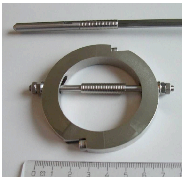
Figure 8. Photograph of the neonatal PS system. The 4 mm pin traverses the 6.4 mm diameter sleeve and is secured to the ring using 4 mm nuts. The ring has an outer diameter of 70 mm and an inner diameter of 50 mm. At the top of the photo, the sleeve is shown mounted onto the insertion instrument.
