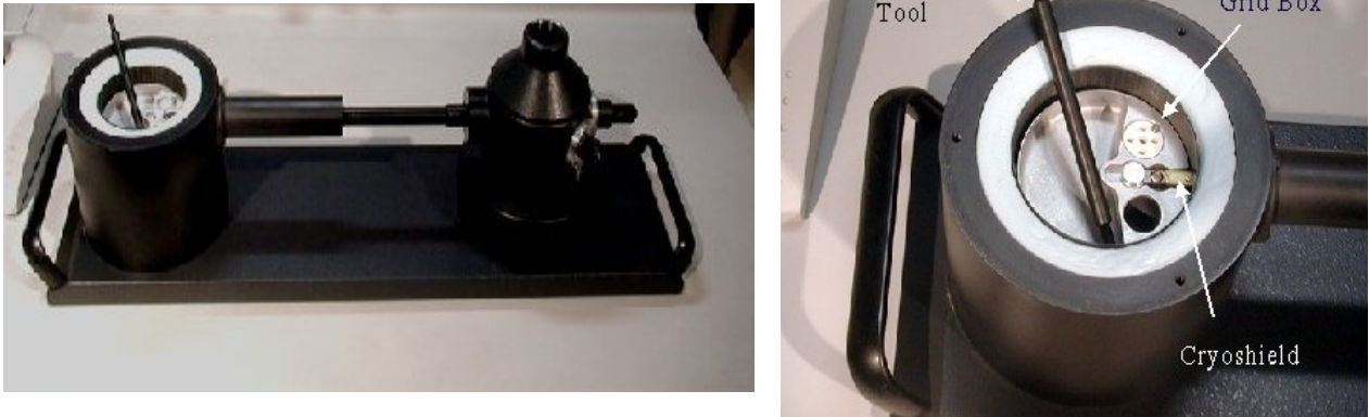
Figure 20 : Photos de la station de transfert (Gatan 626) (FEMR McGill)
