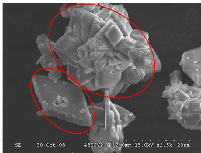
Figure 5.3: SEM images of \text{LiFePO}_4 synthesized using the thermal decomposition of urea under hydrothermal conditions.
