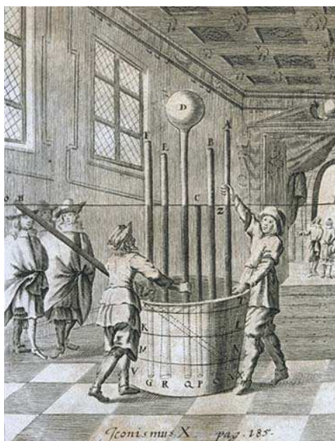
Figure 3.1: The experiment made by Torricelli. Gaspar Schott, Technica curiosa, sive, Mirabilia artis , Würzburg 1664. Source: Institute and Museum of History of Science, Florence, Italy (Source: http://www.imss.fi.it/vuoto/eesper2.html ).
