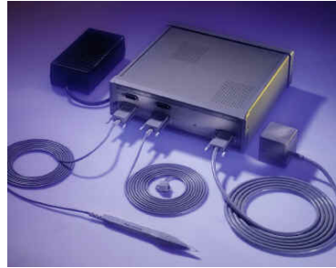
Figure 2.6: AC electromagnetic tracking device by Polhemus (Polhemus Inc., Colchester, USA) 21
