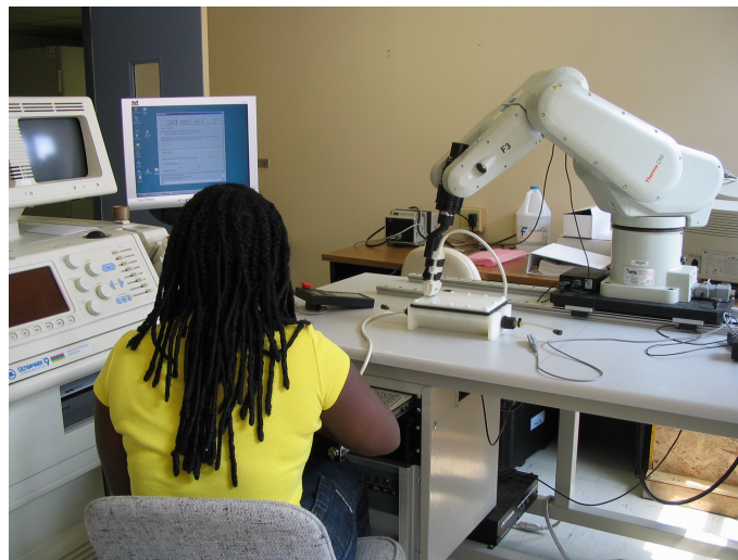
Figure 2.12: The 3D-ultrasound (US) robotic imaging system. The F3 CRS robotic arm carries a probe from an US system (GE Vivid-5).
