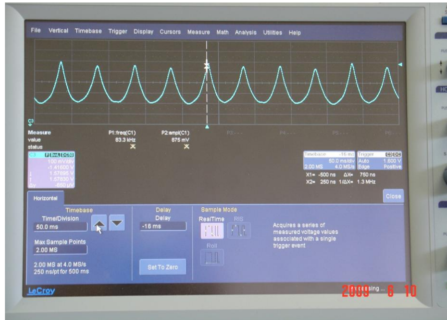
Figure 4: Signal with the new HWP rotating at 300 RPM, at 353 GHz, without the analyzer and the calibrator.
