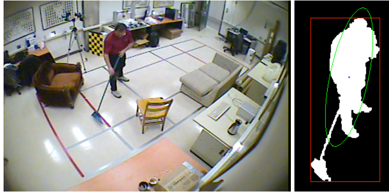
Figure 3.11 – Example of the bounding box (red) and of the approximated ellipse (green) of the silhouette. We can see here that the bounding box is very sensible to carried objects.
