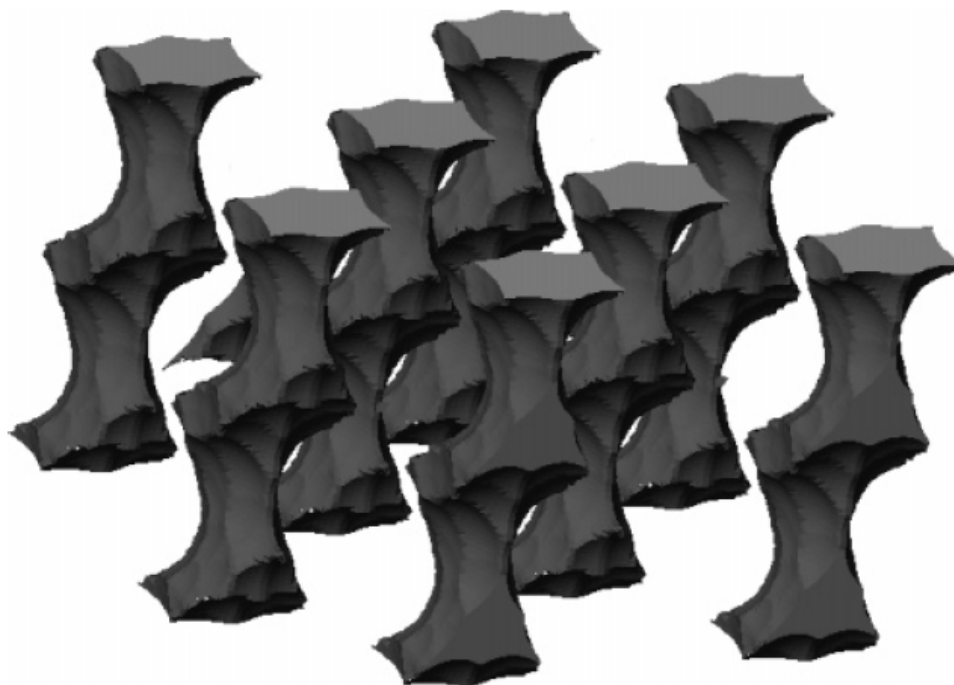
Figure 15. Representation of channels along the c -axis in the network resulting from crystallization of tecton 7 from DMSO/dioxane. The image shows a 2 \times 2 \times 2 array of unit cells. The outsides of the channels appear in dark gray, and light gray is used to show where the channels are cut by the boundaries of the array. The surface of the channels is defined by the possible loci of the center of a sphere of diameter 6 Å as it rolls over the surface of the ordered network. 36
