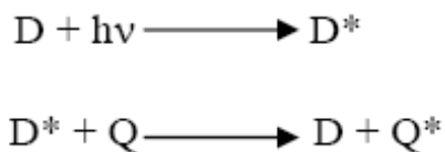
Figure I-7. Quenching of an excited state donor, \text{D}^* , by an acceptor [\text{Q}] .
