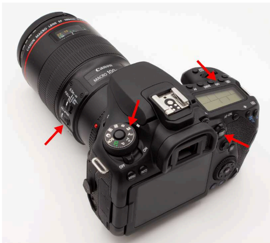
Figure 3.5: Camera (Canon EOS 90D) and lens (EF 100m f/2.8L MACRO IS USM) used to take RAW photos for focus stacking. Arrow on the lens: Focus mode button set to Auto Focus (AF). Arrows on the camera body (from top to bottom): ISO button, Manual Exposure mode dial and “START-STOP” button (for Live View Shooting Mode).
