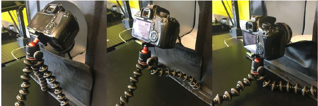
Figure 4.4: The three camera positions from which pictures should be taken for each flower position. Adjust the number of flower positions and number of photos according to each flower. For intricate flowers, or flowers that can't be captured entirely with only two positions (ventral and dorsal), you can place the flower on an another position (Figure 4.3). On the contrary, if the flower can't be placed on several positions, you may need to increase the number of photos per camera height in order to have sufficient information for the software to reconstruct accurate 3D models.
