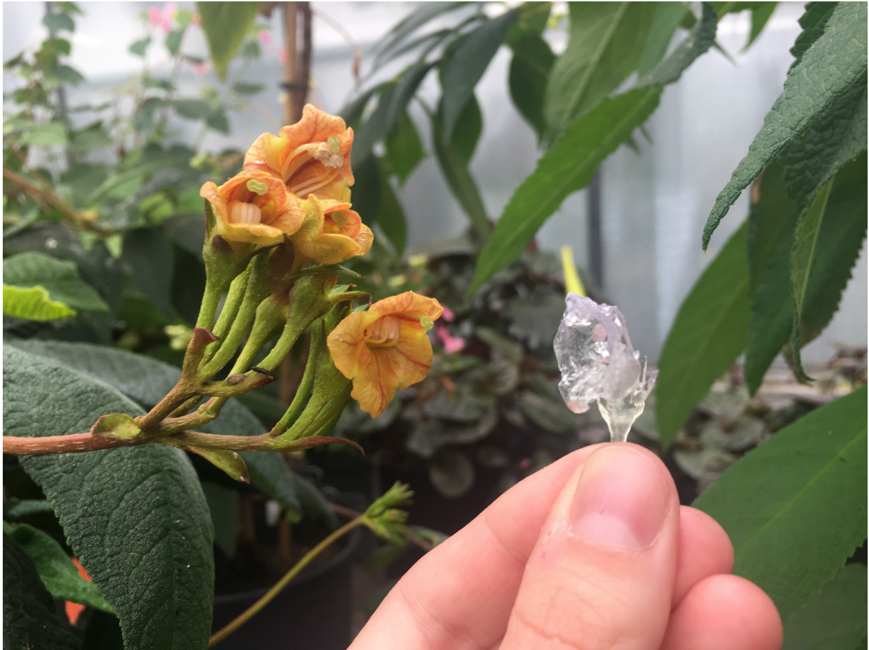
Figure S13. Example of a 3D-printed flower of Gesneria cornuta in clear and soft resin. We used the Form 3 3D-printer from Formlabs (Somerville, Massachusetts, U.S.) to print Gesneriaceae flowers. After they were printed, the models were rinsed in fresh isopropyl alcohol (IPA), the supports used to stabilise the models while being printed were removed, and the final models were post-cured using heat and 405 nm light.
