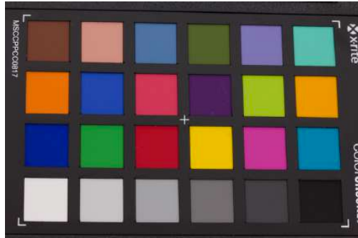
Figure 4.1: Colour chart photo taken at the beginning of the process to calibrate the photos in post process.
