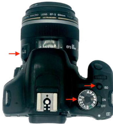
Figure 3.3: Camera (Canon T2i/550D) and lens (60mm f/2.8 Macro lens) used to take RAW photos. The red arrows (from top to bottom) depict the button to get manual focus, the ISO button and the Manual Exposure mode dial.
