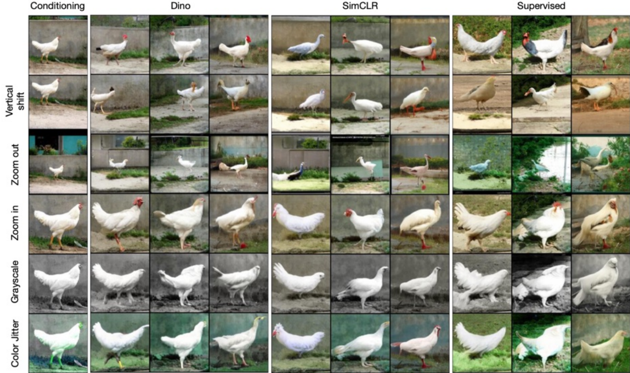
Fig. 3. Using our conditional generative model to gain insight about the invariance (or covariance) of representations with respect to several data augmentations. On an original image (top left) we apply specific transformations (visible in the first column). For each transformed image, we compute the 2048-dimensional representation of a ResNet50 backbone trained with either Dino, SimCLR, or a fully supervised training. We then condition their corresponding RCDM on that representation to sample 3 images. We see that despite their invariant training criteria, the 2048 dimensional SSL representations appear to retain information on object scale, grayscale vs color, and color palette of the background, much like the supervised-trained representation. They do appear insensitive to vertical shifts. We also see that supervised representation constrain the appearance much less. Refer to Fig. 20 in Appendix for a comparison with using the lower dimensional projector-head embedding as the conditioning representation.
