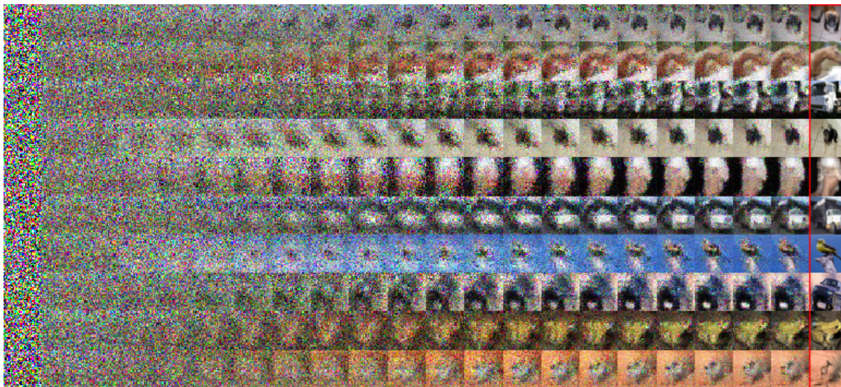
Fig. 5. An example of an infusion chain by Bordes et al. [28]. Starting from noise, we gradually infuse very few target pixels into the sampling chain. By doing so, the network learns to construct back the image gradually. At inference, we remove the infusion steps to sample from the model.
